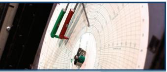
Our comprehensive **Quality Management System** includes full function, hydrostatic and pneumatic pressure testing to prevent defective orifice fittings from reaching service. Standard testing comes at no extra charge and includes verifiable pressurization to 150% of working pressure. Additional inspections, such as radiography, ultra sonic and liquid dye penetration, are also available.
